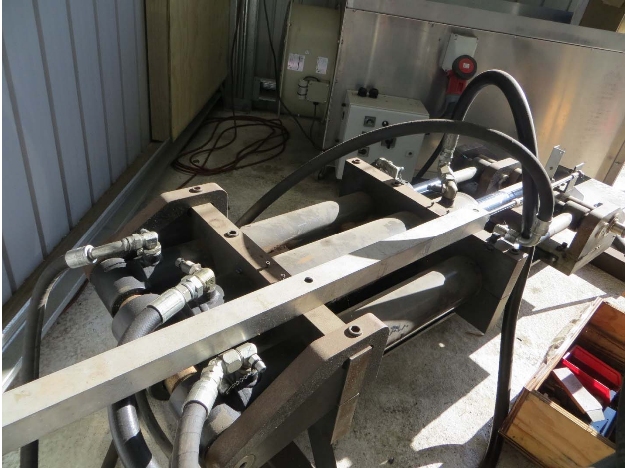
Figure 6 Hydraulic Rig Used to Drive Cylinders out of Power Pod Structure
