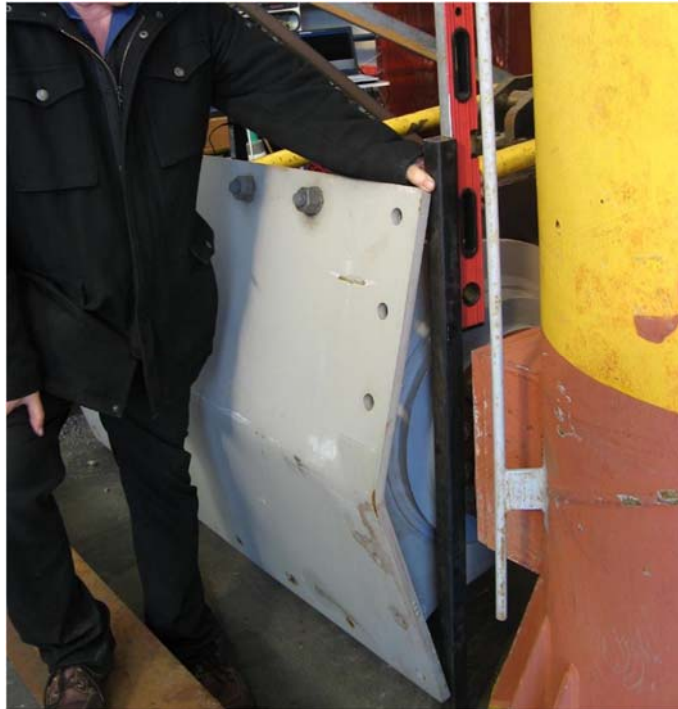
Figure 8-5 Method used to determine zero position of angle sensors
